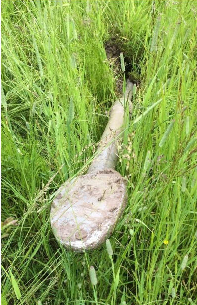
Pilot rod with steering head
