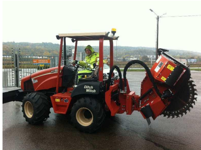
Example of machine with milling wheel
