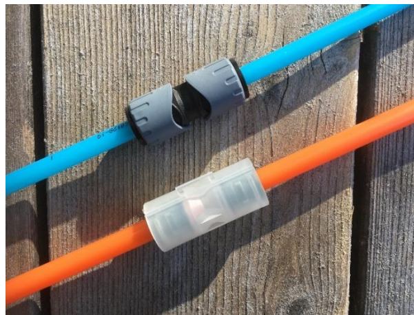
Examples of splicing of microducts
